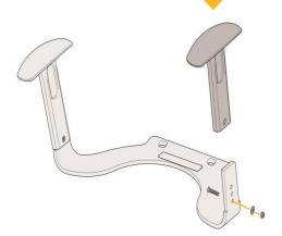
2. Insert the bolts making sure the countersunk heads are located on the inside of the arms and tighten nut over washer. Do not over tighten!
